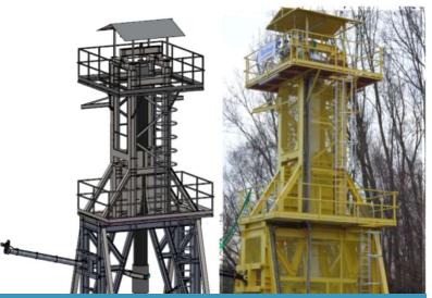
Hydraulic test bench, vertical bending tests on flexible pipes (16 inches 10 meters long): cryogenic fatigue test on controlled pressure
