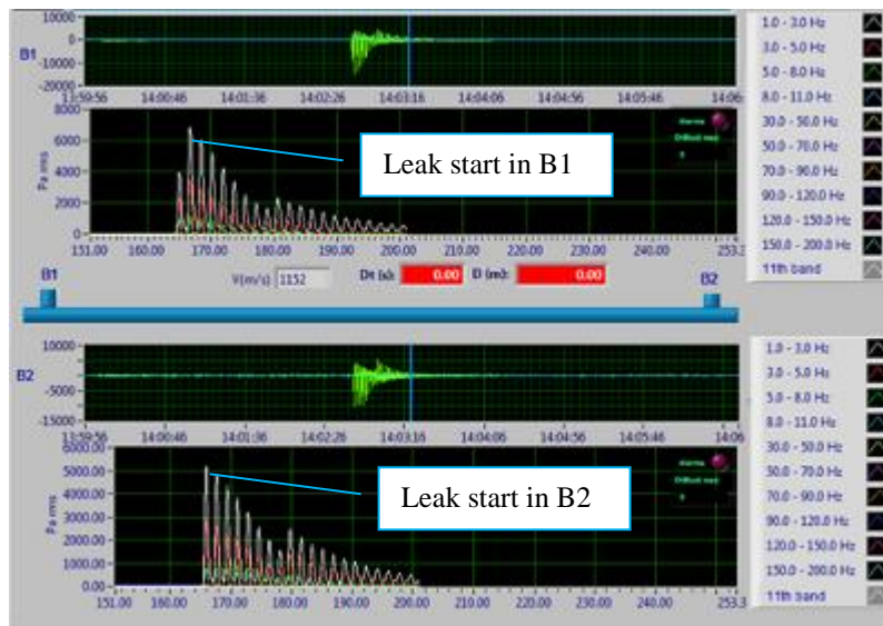
Fig. 22: Detection and localization of leak using frequency bands
