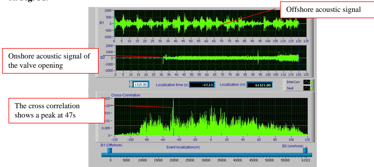
Fig. 31: Leak Start analysis by cross correlation
