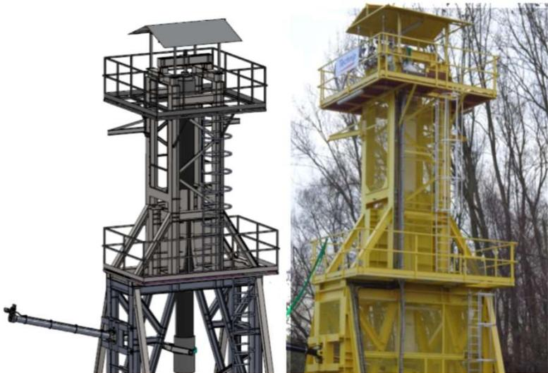
Hydraulic test bench, vertical bending tests on flexible pipes (16 inches, 10 meters long): cryogenic fatigue test on controlled pressure
